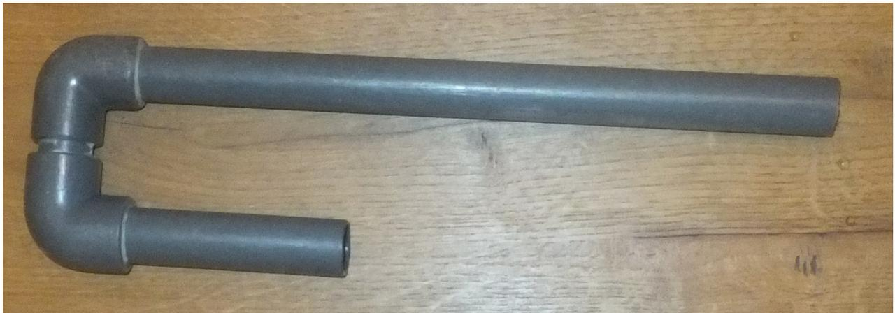
A U-bend is made of GF pipe and has two 90° GF joins (elbows). They are available in stores which stock plumbing supplies. Using a U-bend has the advantage that you can regulate the amount of water that will drain from the aquarium via changing the length of the shorter arm of the U-bend. This also prevents your aquarium from accidentally draining completely! (PHOTO: U-bend)
